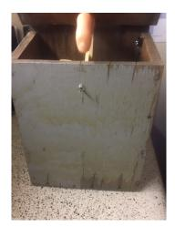
**4.** Finger flips toggle switch back to OFF (notice momentary switch on the right is open, allowing electricity flow through system)
