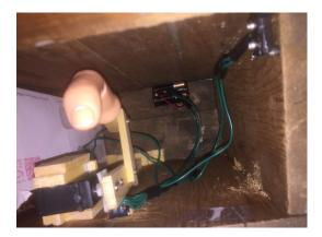
(wire connections between the battery holder, toggle switch, servo motor and momentary switch is made.)
