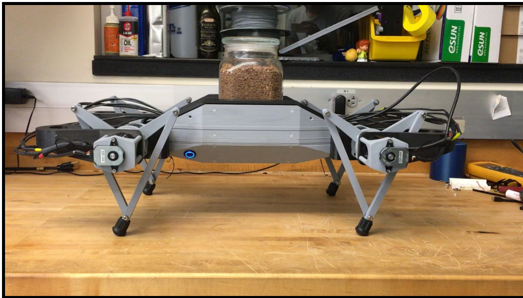
Figure 4.8. Carrying Capacity Test (Using measured amount of sand as additional weight)
