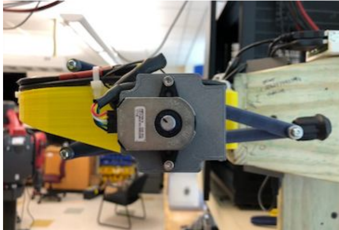
Figure 4.11. Correct shaft position of the outer motor after calibration.
