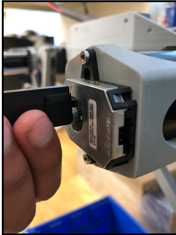
Figure 4.2. Measurement of Shaft of the Encoder
