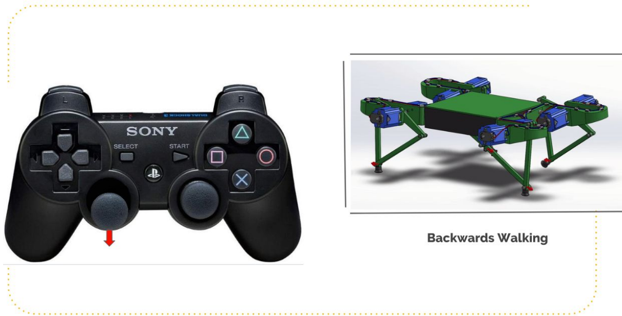
Figure 3.6. Backwards walking of robot with controller input shown.
