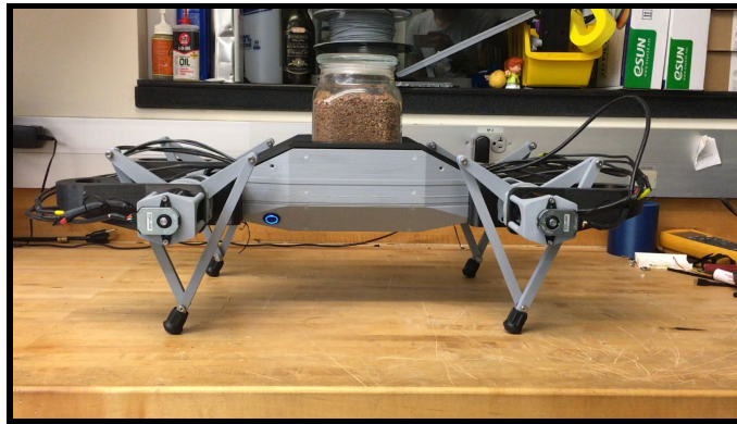
Figure 5.2. Weight Carrying Test being Conducted
