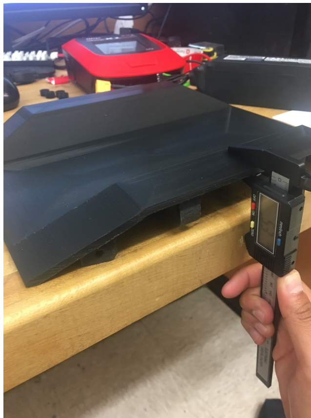
Figure 4.5. Thickness of the Cover
